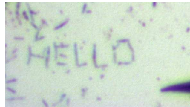
10-20 \mu\text{m} long, 250nm wide polymer sticks being manipulated
